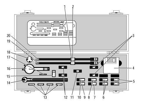
Figure 1-5. Model 3654 (V Connector) Calibration Kit Components
